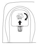
9) Flip the retainer from front to back, then slide it back into the slot so that the lip of the retainer faces up and the oval is at the bottom of the retainer. This will hold the handset in place.
